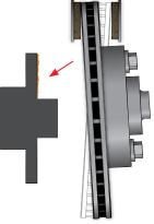
Although we are unable to change the habits of a consumer there are steps that can be taken to minimise the formation of corrosion. At the point of installation, cleaning the hub surface and protecting with a suitable lubricant will prevent corrosion build up.
