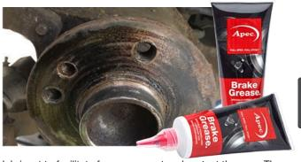
lubricant to facilitate free movement and protect the area. The lubricant used must be able to withstand high temperatures and must be completely metal free to avoid galvanic corrosion that will restrict movement. Apec Braking provide a petroleum-based lubricant that effectively protects surfaces as well as being fully compatible with ABS and ESP braking systems.
