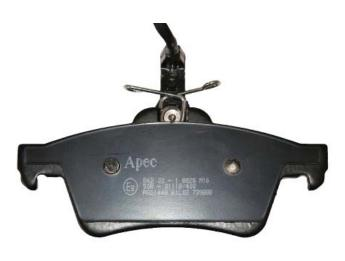
Insert the spring and wear sensor back it to the pad using a suitable tool.
