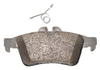
To correctly fit the wear sensor, first remove the pad spring fitting from the top of the pad using a suitable tool.
