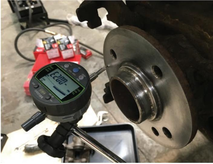
measurement of the hub was taken. The maximum amount of tolerance for the hub runout is  $>0.04\text{mm}$ . The nearside hub gave a runout measurement of  $0.08\text{mm}$ . As the hub was distorted it was causing the brake disc to be misaligned when it was fitted, hence affecting the even material transfer process, gradually causing the brake disc to develop excessive DTV and manifesting itself into a
