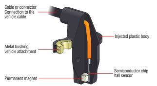
There are two types of active sensor. The Hall sensor and the Magneto-resistive sensor.
