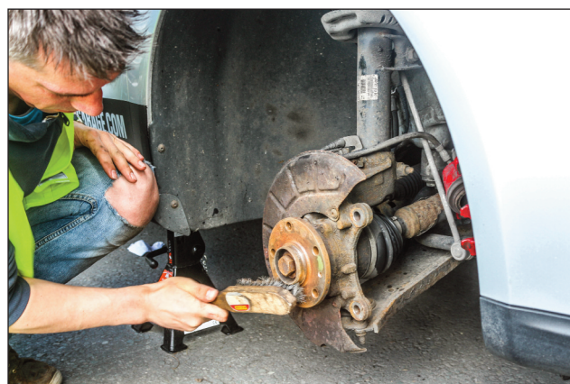
Remove all of the contact and surface rust from the hub
