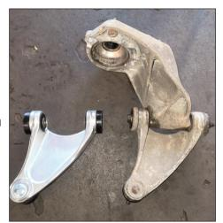
The top arm assembly needs to be completely removed from the vehicle before the retaining bolt can be removed
