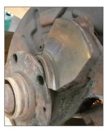
The brake pad surface was larger than the braking surface area of the disc allowing the strange wear
