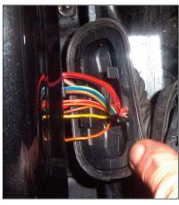
The wire beneath the rubber boot had failed between the door and body
