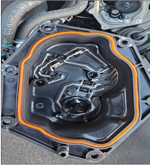
This Audi Q5 has a well known corrosion fault, when moisture enters the electronics of the EGR Valve
