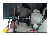
tools, in order to prevent the piston jamming or twisting.
