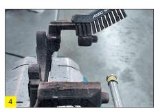
shafts of the dismantled caliper bracket using a wire brush and/or caliper file.
