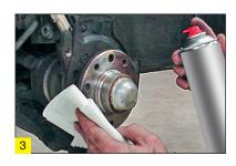
We recommend checking the cleaned hub with an appropriate measuring gauge (measuring dial with stand) for possible lateral run-out and other possible deviations.
