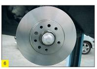
We recommend measuring the newly fitted brake discs for lateral run-out approx.15 mm below the maximum radius using a dial gauge. Ideally, this measurement is performed with a properly mounted wheel.
