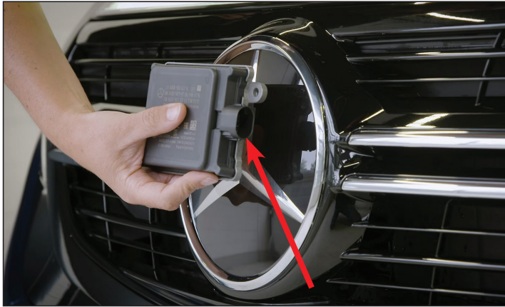
The DISTRONIC unit is located behind the grille
