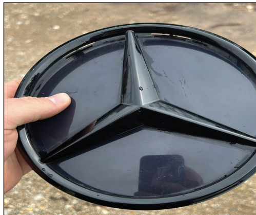
The grille was painted black, disturbing the DISTRONIC unit function
