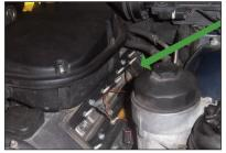
The rear plug on the nearside bank is the most difficult to replace
