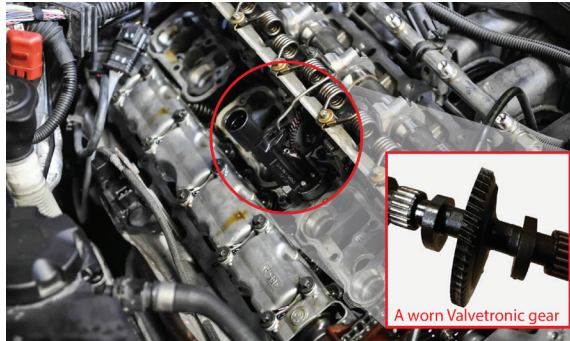
A worn BMW Valvetronic shaft component or a faulty stepper motor are the most common causes of failure
