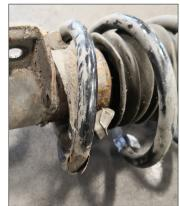
When the smaller lower coil spring fails the suspension can drop leaving the vehicle immobile the circumference of the main body of the spring. This means that if the spring breaks at the end coil (and they do) the rest of the spring will go flying past the contact point.
