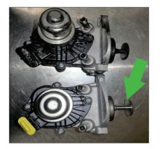
It is important that the valve is powered into the energised position to prevent contact when fitting
