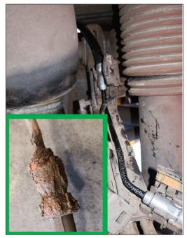
The BMW hadn't travelled far but that didn't stop the corrosion from getting into the brake pipes
