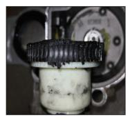
The nylon drive gear had stripped and was no longer driving the transfer control
