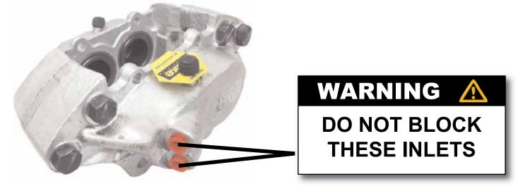
The above calipers are all 2 inlet fitting and must <u>NOT</u> be fitted to 1 inlet applications. By blocking one of the inlets braking efficiency will be considerably reduced, as only two of the four pistons will be working.
