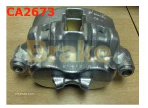
CA2673 Brembo/Iveco Piston Øs = 52 mm Pad Gap = 76 mm Bleed nipple angle = 15°
