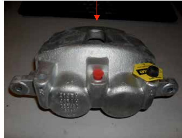
CA2743 Kelsey Hayes Slider Ø = 10mm Pitch = 204mm (Centres) Jeep is embossed on outer face
