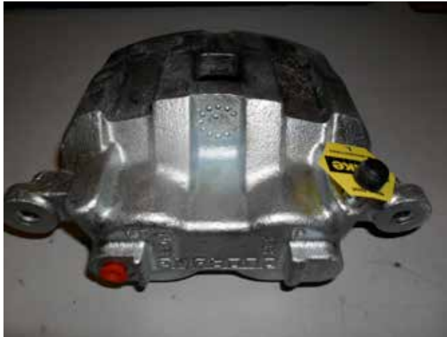
CA2358 Akebono Slider Ø = 8mm Pitch = 190mm (Centres)
