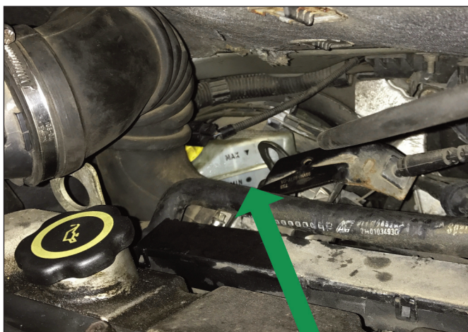
The brake master cylinder and reservoir are hiding deep in the engine bay, making topping up very difficult
