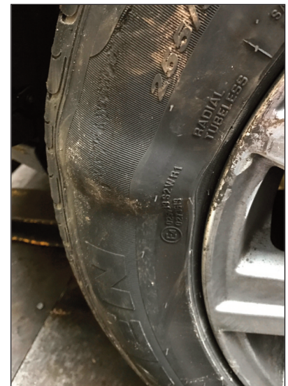
The bulge in the tyre made it unfit for purpose even though it was less than a month old
