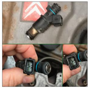
The leaking washer jet had allowed the corrosive washer fluid to enter the injector plug damaging the terminals
