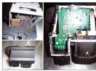
The fan running constantly and then its failure was due to the water which had penetrated the control module
