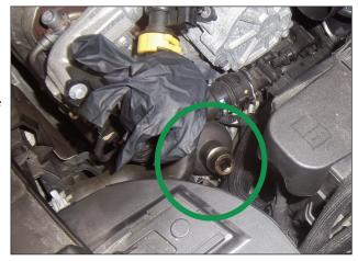
Access to the housing first requires the induction hoses to be removed, note we have covered the opening to the turbo with a glove for safety
