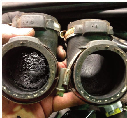
One side of the twin EGR system on a TDV8 Range Rover was treated with Revive, leaving it cleaner than the side on the left
