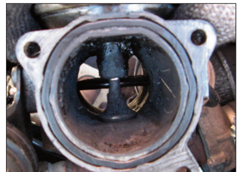
A fouled EGR Valve, above, and the same valve, below, after it was cleaned with JLM EGR Valve Cleaner, available from Breen Distributors, Kanturk. After cleaning the EGR valve, look for other faults that could have caused the fouling
