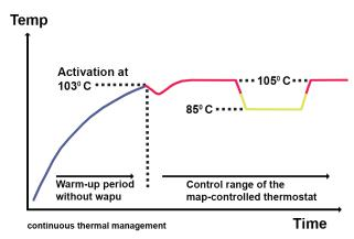
Moreover, in addition to creating the on-demand water pump, the engineers have developed a map-controlled thermostat that completes the thermal management system. In order to optimise the volumetric efficiency and avoid knocking, this allows the engine to run at a coolant temperature of 105 °C when working at part throttle and of 85 °C when working at full throttle.
