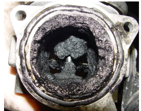
An EGR Valve this heavily fouled will not be capable of working correctly, but after cleaning it may be fine
