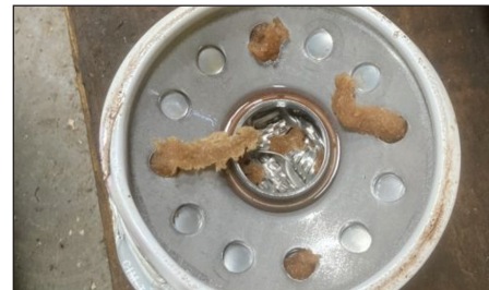
Some examples of the build-up of fatty acids in the fuel filter
