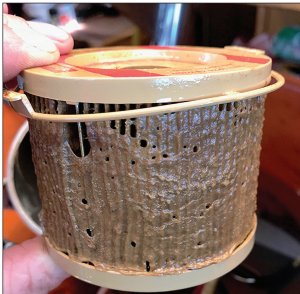
Some examples of the build-up of fatty acids in the fuel filter
