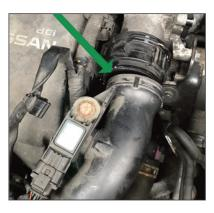
The intercooler pipe had split at the top of the engine where it joins onto the connector
