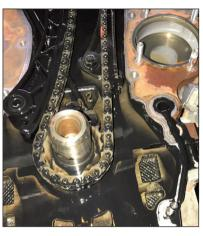
After a short test drive, I decided I needed to check things out a little closer and set about checking the valve timing. Sure enough, the timing was out a little. I suspected that not long before he had purchased the van, a new timing chain had been fitted. It had either not been set up correctly, or the crankshaft pulley hadn't been tightened to the correct torque.
