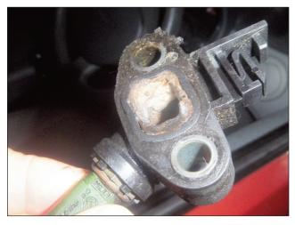
The leak was from the small outlet which also houses the coolant temperature sensor
