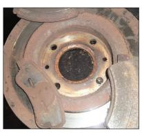
Corrosion had really taken hold and the brake discs and pads were good for nothing but the bin
