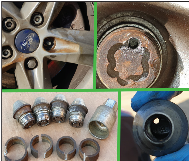
A hole drilled in a strategic position can often ease the removal of a stubborn nut
