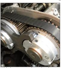
With the correct tools, setting the timing and fitting the new belt on the variable valve timing engines is slightly quicker
