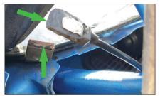
The connection on the terminal is quite a common failure
