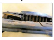
The friction plate had ripped away from the centre spline, allowing it to spin freely
