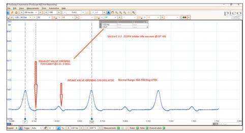
In-cylinder pressure showed the exhaust valve was opening too early because the chain had jumped
