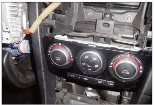
The radio and lower trim panel require removal, to access the fittings for the control unit
