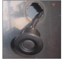
Failure of the boot operating button is easily fixed by replacing the button
