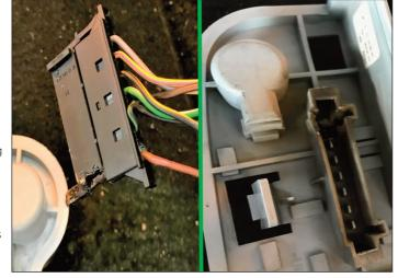
A poor connection in the plug caused the terminal to heat up and accelerate the problem
