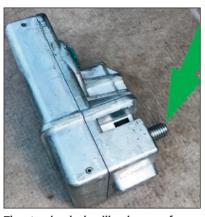
The steering lock will only come free of the column by pushing the threaded fixing into the lock, this can only be done in the unlocked position
