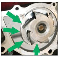
With the pump removed the wear on the body from the impeller could be seen, this was the source of the noise
