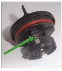
The contact point on the bulb holder had burnt through due to a poor contact
