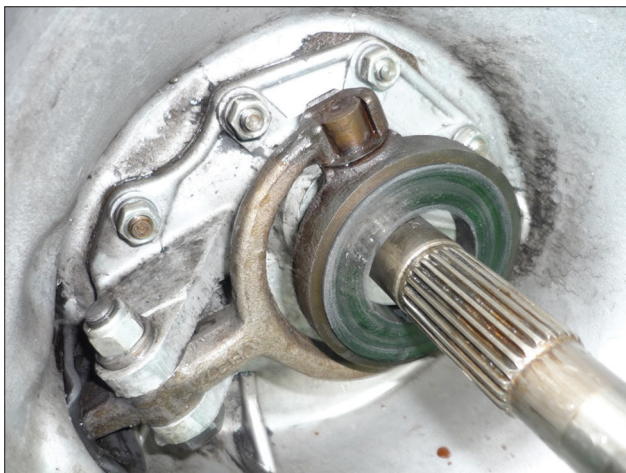
The carbon thrust release bearing had worn down
