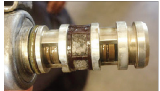
Contaminated filter screens like this can seize the solenoid and cause low engine oil pressure
