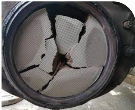
Internal damage to a DPF will trigger errors and may prevent proper operation
