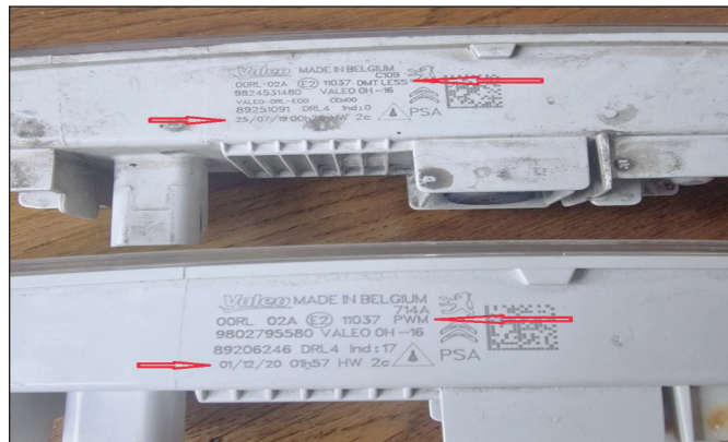
The DRLs looked identical, but were not compatible as a pair as one was marked "PWM" and the other was marked "DMT Less"
