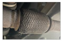
An air leak in the exhaust flexible pipe was distorting the emissions
