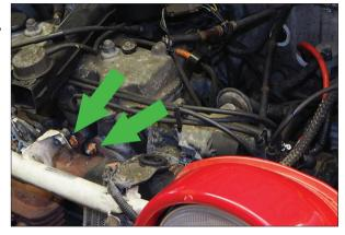
Fitting new nuts and studs when reassembling should hopefully ensure that the next time the manifold needs to be removed, the job will go smoothly
